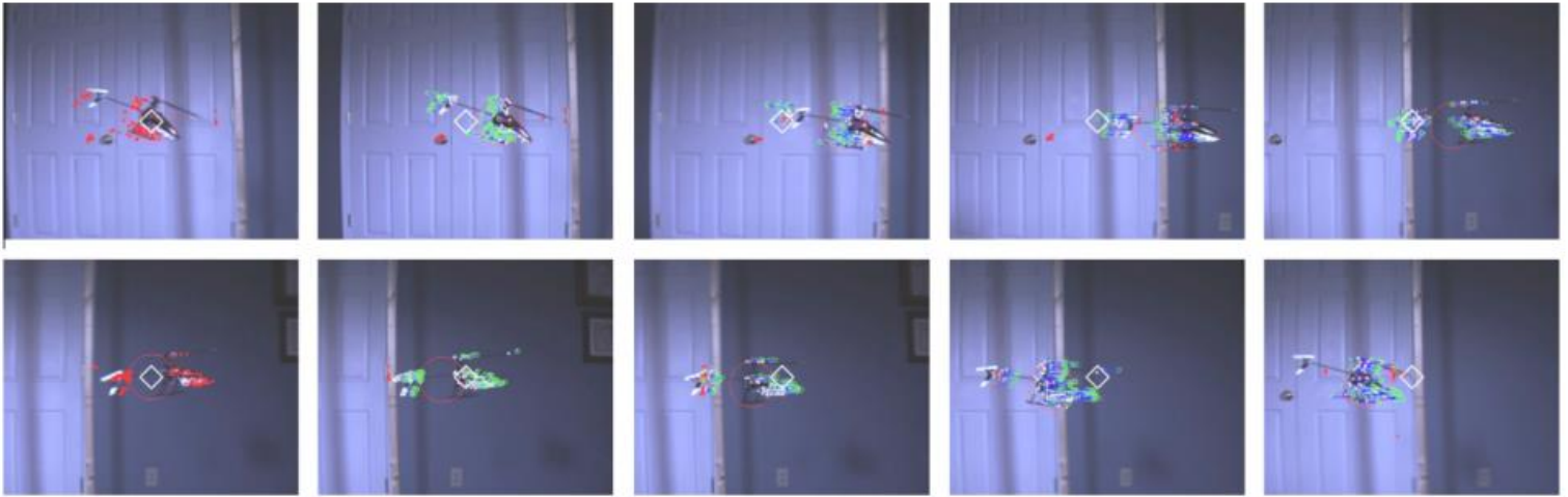
Fig. 12. A sequence of frames, approximately 0.24 s apart for one period, of a swinging SUT with the center of the image identified by a white diamond, previous points shown as green rectangles, g_{i-1} , current optical flow points as white, closed circles, g_i , estimated points as green, open circles, \hat{g}_i , and removed outliers shown as red, closed circles. (For interpretation of the references to color in this figure legend, the reader is referred to the web version of this article.)
